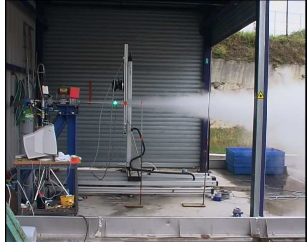
Figure 6. PDA droplet size measurement for large-scale butane jet experiment (INERIS)
