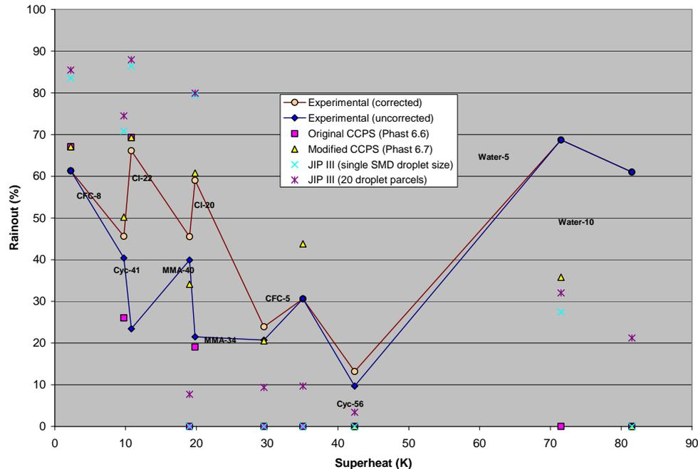
**Figure 9. Validation of rainout model against CCPS experiments**
