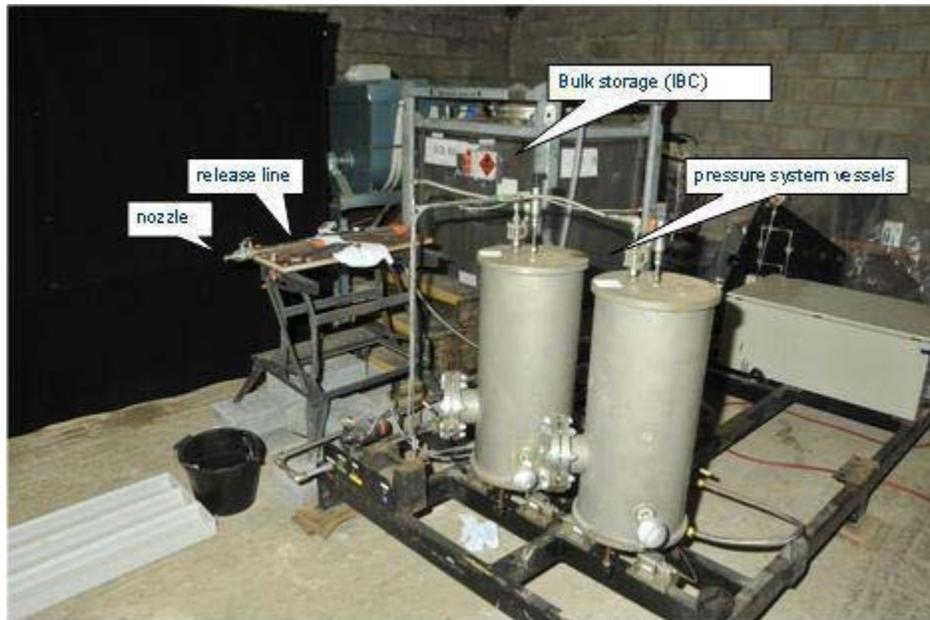
**Figure 2. Experimental rig**
