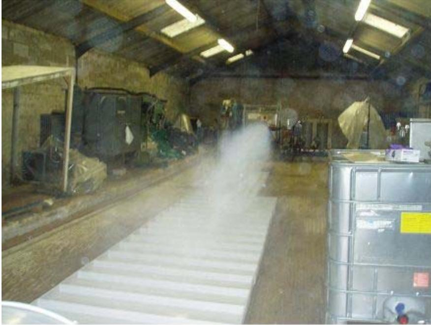
**Figure 4. Distributed rainout measurements**
