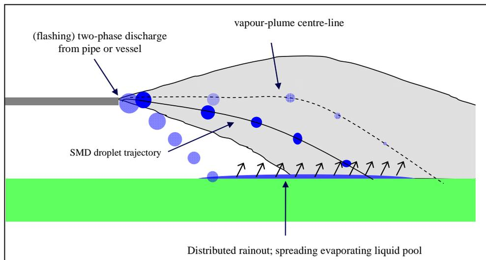
**Figure 1. Discharge, droplet dispersion, distributed rainout and re-evaporation**
