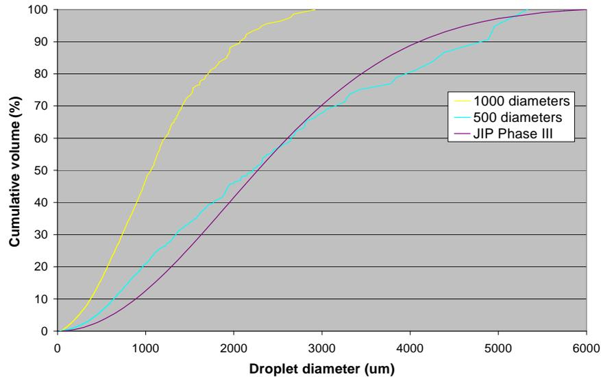
**Figure 6. Validation of droplet size distribution (water experiment, 2.5mm nozzle, 10barg)**
