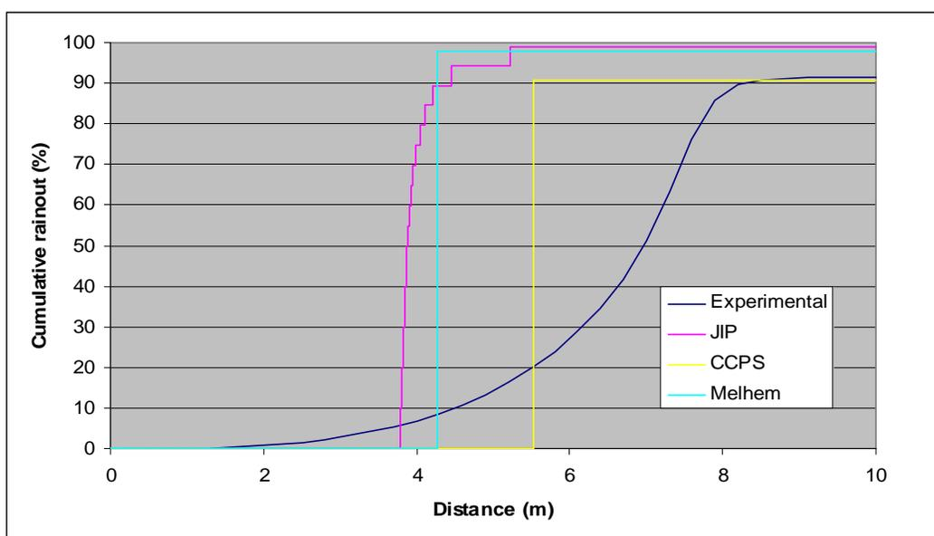
Figure 8. Validation of rainout model against HSL xylene experiment (2.5 mm nozzle, 8 barg)
