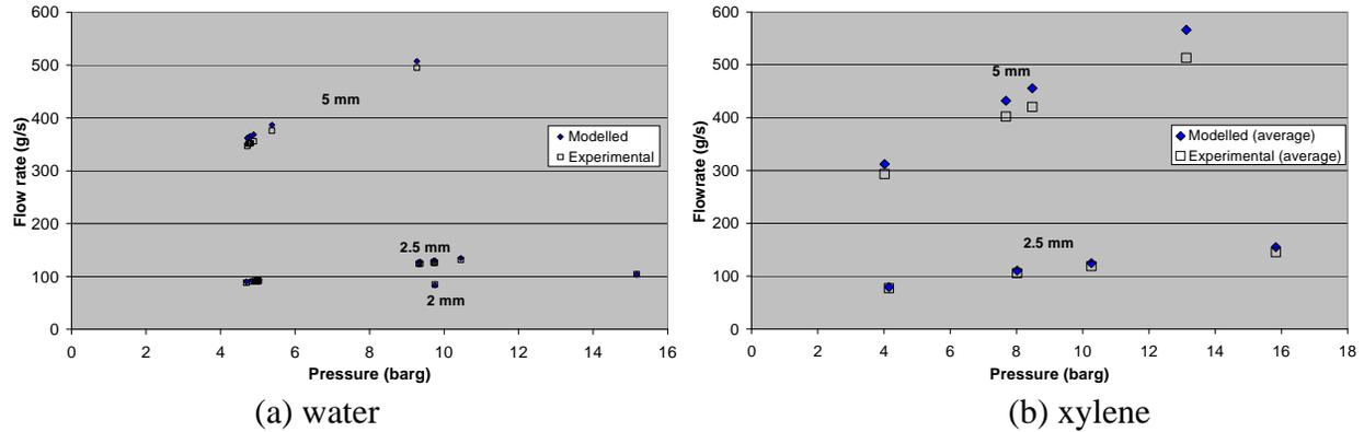
Figure 5. Validation of flow rate for HSL water and xylene experiments
